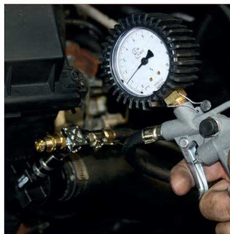
**Turbocharger charged air system inlet test adapter, bayonet**
