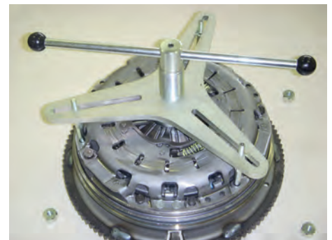
15. Loosen hexagonal nuts - remove clamping device.
