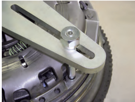
11. Screw on hexagonal nuts by hand until these are flush with the threaded bolts (parallel mounting of the SAC clutch tool set). Attention: The pressure spindle must be completely screwed back.
