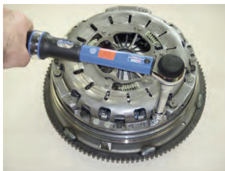
17. Screw the missing cover fastening screws into the now free threaded receptacles on the flywheel hand-tight. At the end, tighten all fastening screws with the torque stipulated according to the manufacturer's specifications.
