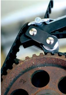
GM / Opel cam shaft locking tool
